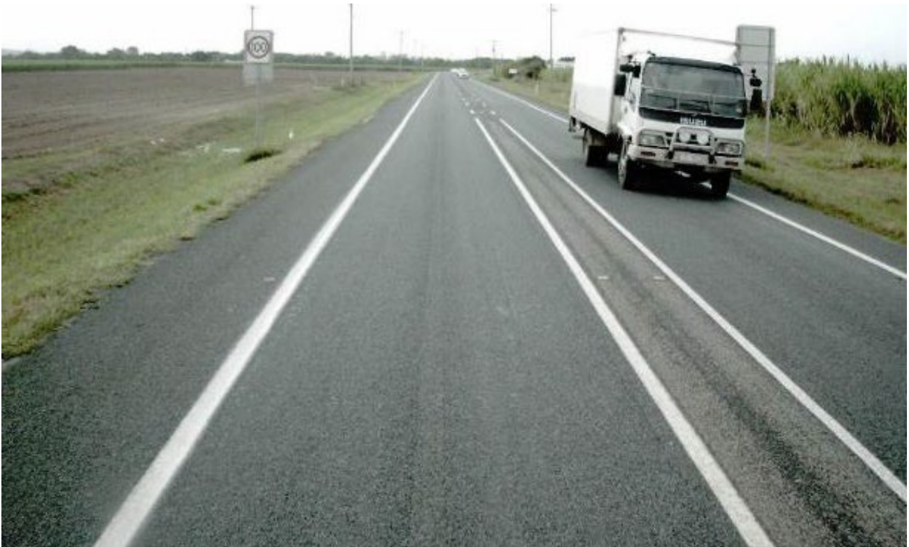
Figure 5.2: Wide centreline incorrectly interpreted as a narrow lane by machine vision
